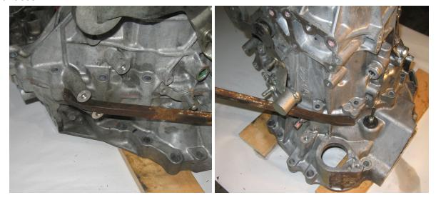
Applying gentle force at these two locations should allow the seal to be broken on the case. If there is resistance make sure you verify that all 17 case bolts have been removed.
