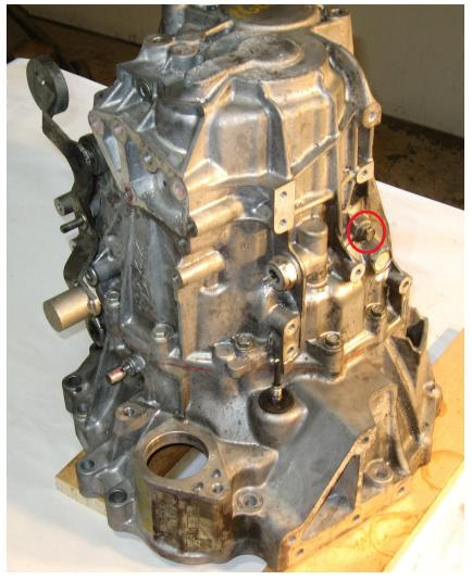
Note that this bolt has a crush washer on it, this bolt needs to go back in the same location on reassembly.
