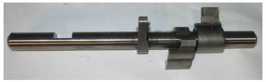
The parts are retained to the shaft with a roll pin, using a punch and a hammer remove the bracket to the left as well as the old cross gate cam.
