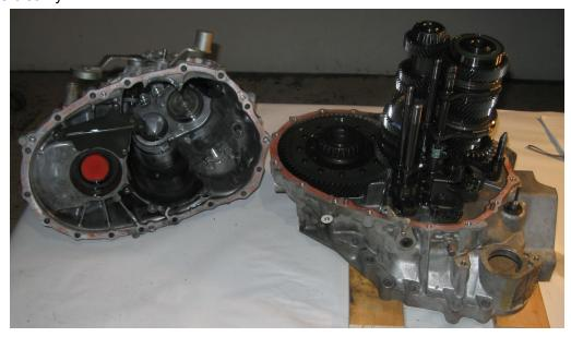
Note that the input shaft (on left in picture) has an end bearing shim that normally stays in the top half of the case. If it did not stay with the top half of the case please put it back in that part of the case.
