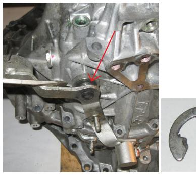
Once that is removed push the shaft into the transmission to collapse the space that was maintained by this e-clip.
