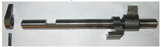
The new cam can then be reinstalled as well as replacing the left bracket back on. Simply gently hammer the roll pins back in place to lock everything back to the shaft.
