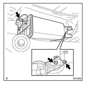
(f) Remove the 2 bolts, clip and charcoal canister.
