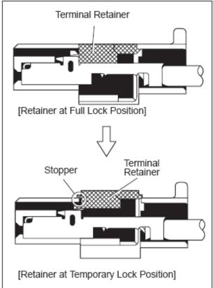
Once the secondary lock is disengaged, the retainer on each terminal can be disengaged to remove one wire using the following instructions.
