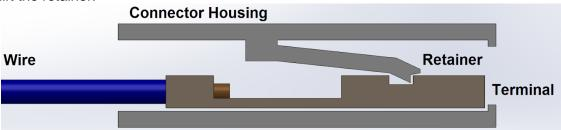
1) Place the tool in the small opening between the terminal and the retainer, being careful to align the chisel point as indicated by the picture:
