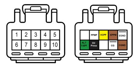
All 22 of these wires should get labeled by function and depinned from the scion TC housings in preparation for insertion into the Spyder's connector housings.
