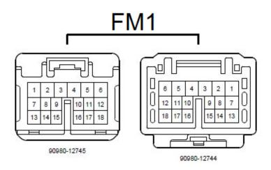
FM1 is the chassis integration connector that is being fitted to the 3<sup>rd</sup> gen Sienna wiring harness to convert it for engine swap use. This fits the pins on the existing harness and can be added with no wire crimping necessary.
