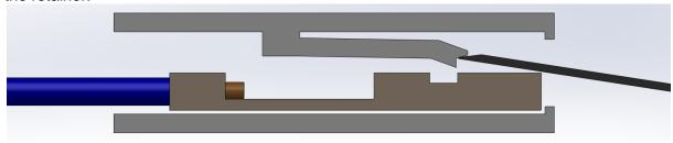
3) Pull on the wire gently to remove it. There should be no resistance to removing the wire and terminal. If there is resistance it is likely the retainer or secondary lock is not fully disengaged. Push the wire back in and go back to the start.
