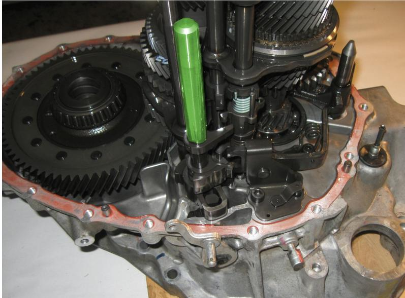
To remove this shaft you need to rotate it clockwise as far as it will go, it will be necessary to lift the shaft slightly while trying to rotate the shaft in order to align all the gates. Once the end is reached it should be possible to jiggle it and lift it away from the rest of the mechanism.
